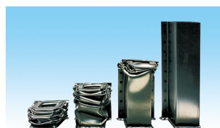
Drop impact test (the middle two products are high-tensile-strength steel materials)
