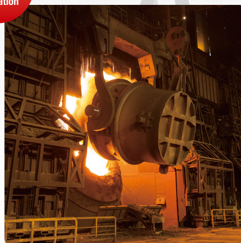
Preliminary dephosphorization and decarburization can be done in a single converter
